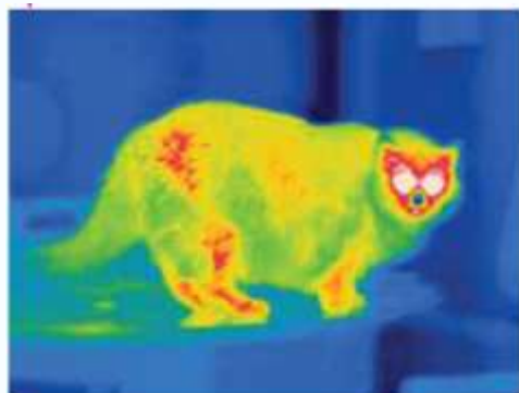
Fig. 18-20 A false-color thermogram reveals the rate at which energy is radiated by a cat. The rate is color-coded, with white and red indicating the greatest radiation rate. The nose is cool. ( Edward Kinsman/Photo Researchers )
